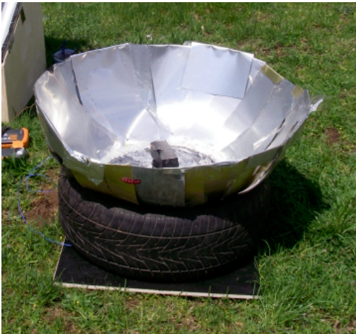
Fig. 7 Tire hybrid cooker
